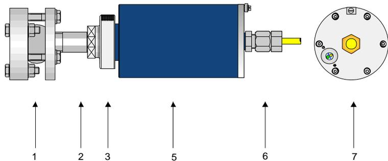
3. with quick release lock and purge air connector
